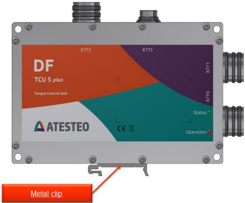
Figure 12 Mounting of TCU5 (with clip)
