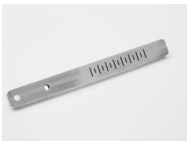
Figure 4 Spline (3x bended with 10°, 3x not bended)
