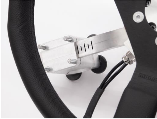
Figure 14 View onto a mounted clamping set on a spline
