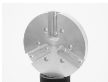
Figure 3 Connector disk (attached to the torque sensor)
