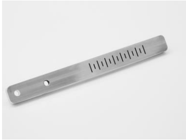
Figure 4 Spline (3x bended with 10°, 3x not bended)
