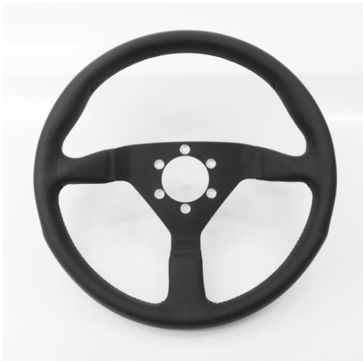
Figure 7 Steering wheel without airbag for attachment to torque sensor
